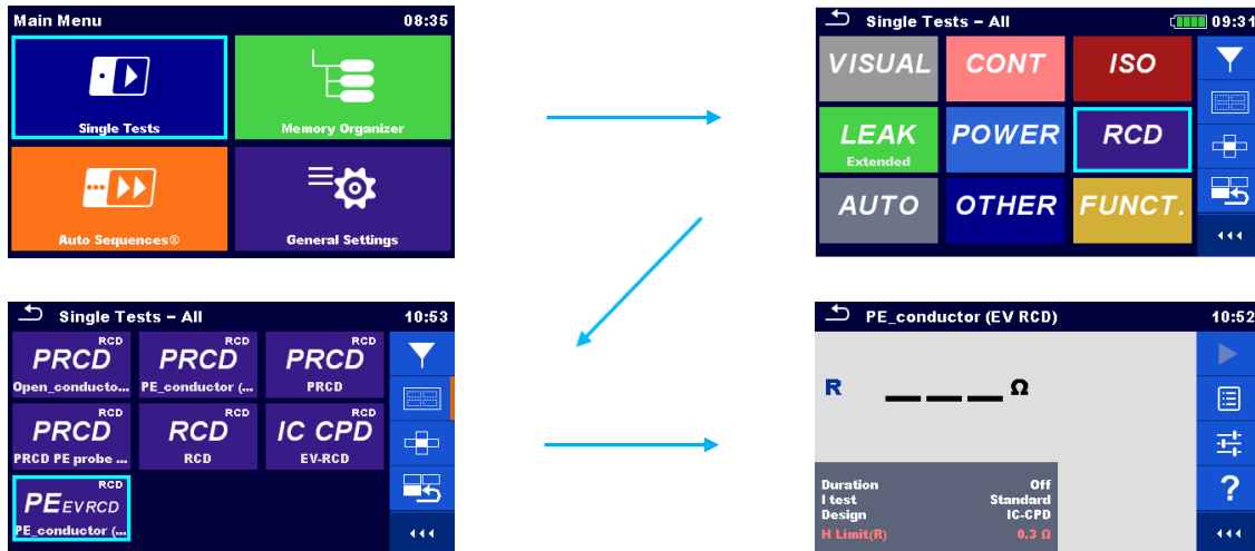
Figure 64_Earth continuity setup
