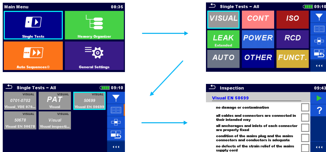
Figure 82_Visual inspection setup
