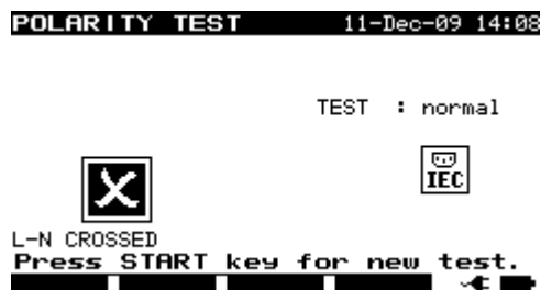
Examples of polarity test result
