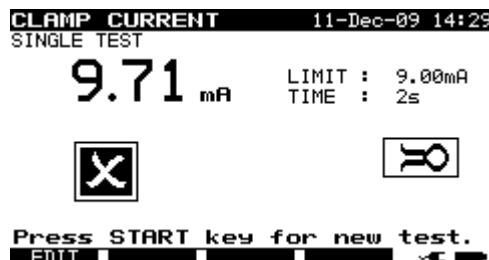
Examples of clamp current measurement result
