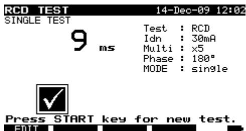
Examples of RCD test result
