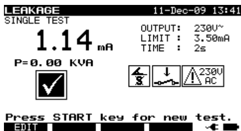
Examples of differential current measurement result
