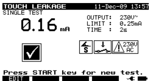
Examples of touch leakage current measurement results
