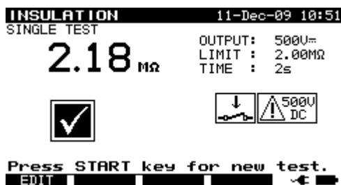
Examples of insulation resistance measurement results
