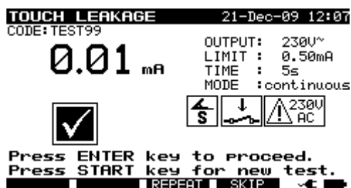
Touch leakage test menu
