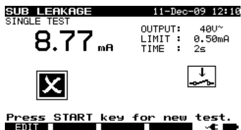
Example of substitute leakage current measurement results
