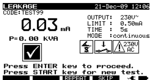
Leakage current test menu
