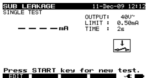
Sub leakage menu
