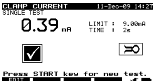
Examples of clamp current measurement result
