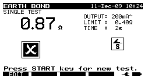
Examples of earth bond resistance measurement results
