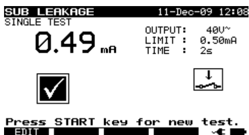
Example of substitute leakage current measurement results
