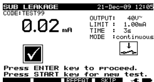
Substitute leakage test menu
