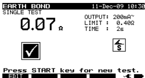
Examples of earth bond resistance measurement results
