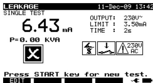
Examples of differential current measurement result
