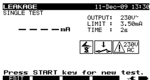
Differential leakage current menu
