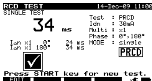
Examples of RCD test result
