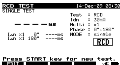
RCD test - single test menu
