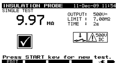
Example of insulation-S resistance measurement results
