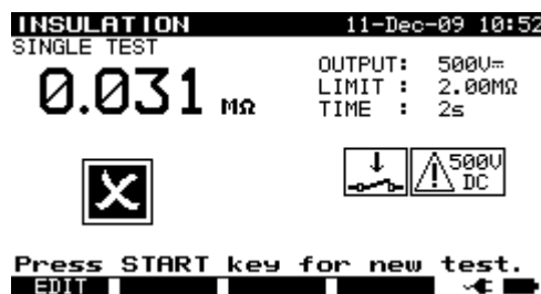
Examples of insulation resistance measurement results
