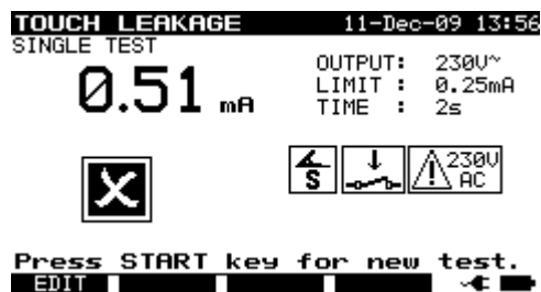
Examples of touch leakage current measurement results
