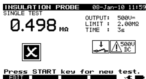
Example of insulation-S resistance measurement results
